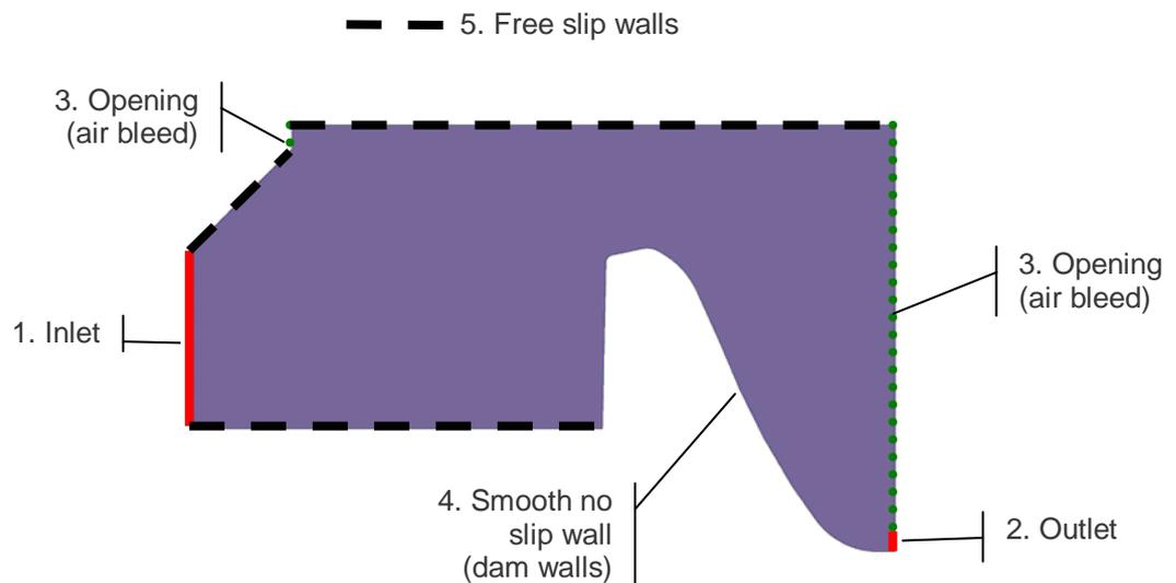
Figure 2. Model domain and boundary conditions
