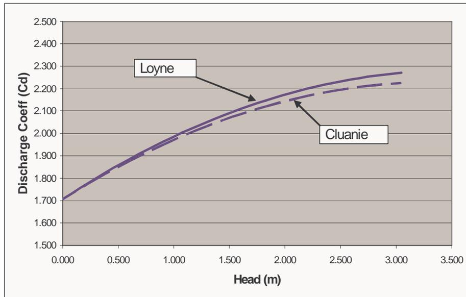
Figure 4. Derived discharge coefficients plotted against head
